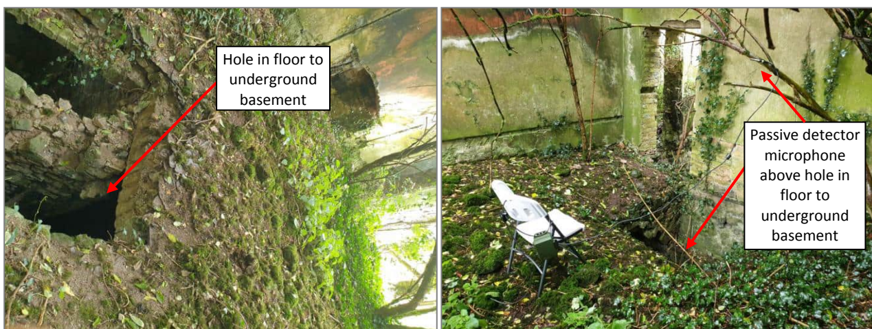
Plate 1. Position of detector microphone in ground floor of Rosmead House ruins above a hole in the floor leading to a permanently dark part of the underground basement
